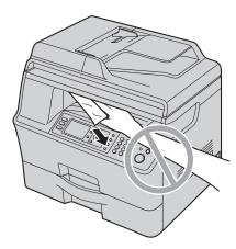
Do not open the paper input tray before opening the left cover as the jammed paper may be pulled and the jam may get worse.
